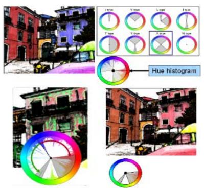
Figure 4. This image (curtsy of Cohen-Or.) represents the different steps of the model provided by Cohen-Or *et al.*. First step consists in finding the closest template from the picture's histogram. Then the hue of pixels which are not in the harmonious areas, is modified accordingly
